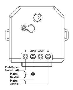
It is normal for any dimmer to produce small amounts of audible noise or buzzing. The noise may vary according to the dimmer setting. Incompatible load types: Ceiling sweep fans, exhaust fans and non-dimmable light sources
